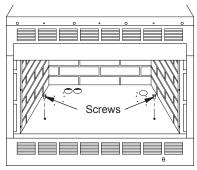
Figure 8 - Removing Screws from Firebox Bottom
